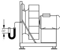
The fans are equipped with a flow measuring device as standard. With the flow measuring device it is possible to measure/monitor the flow easily after the fan is installed.
