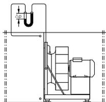
When fans are built in a plenum, it is required to measure the differential pressure between the static pressure in the plenum on the suction side and the pressure at the inlet cone.
